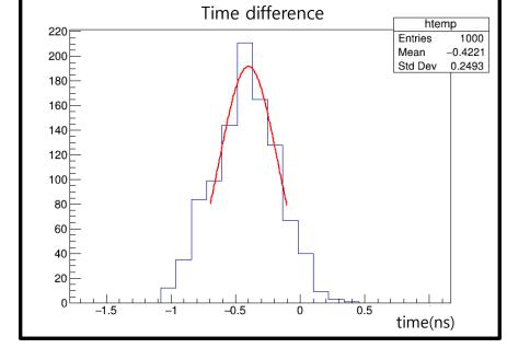
timing resolution  $\sim$  110ps (220ps  $\div$  2) The mean was shifted due to the asymmetry of the location of Am-241 source.
