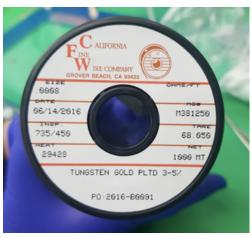
Wire thickness : 16 μm Gold coated tungsten wires for signal and potential wires
