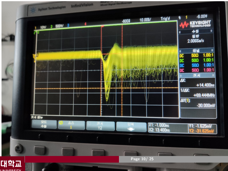
Figure: Gain at last OpAmp is X3
