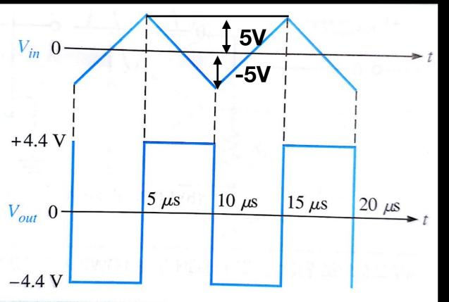
$$I_{C} = \left(\frac{V_{C}}{t}\right)C; \quad V_{in} = V_{C} - 0$$
