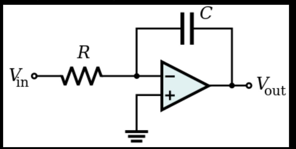
For ideal OP Amp. Input impedance :  $\infty$ Input current : 0 Input offset voltage : 0
