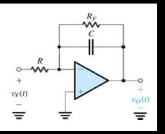
Offset problem is solved by connecting a resistor in parallel to the capacitor.
