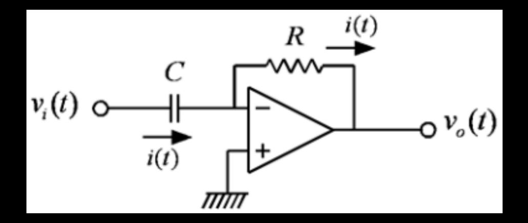
For ideal OP Amp. Input impedance :  $\infty$ Input current : 0 Input offset voltage : 0  $V_{-}$  &  $V_{+}$  are virtually grounded
