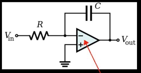
$$\frac{V_{in} - 0}{R} = C \frac{d}{dt} (0 - V_{out}) \quad (\because V_{-} = 0)$$
