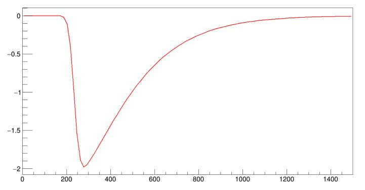
• Single photon signal for MPPC used in DCV
