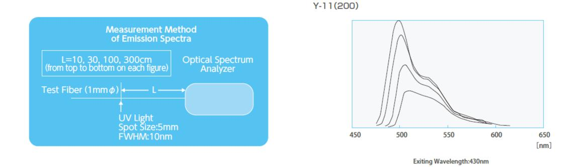
When photon of a wavelength of 430nm shoot in the end of fiber, the emission spectrum should be same as the right.
