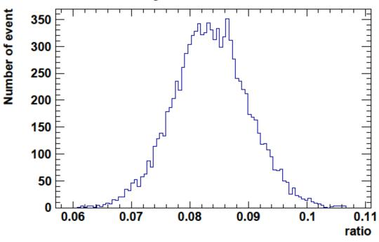
Ratio between the number of WLS process and the number of photon arrived at MPPC
