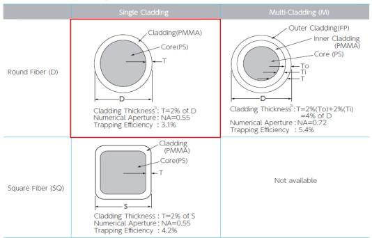
1) In some cases, cladding thickness T is 3% of D. 2) In some cases, cladding thickness T is 6% of D, To and Ti are both 3% of D.
