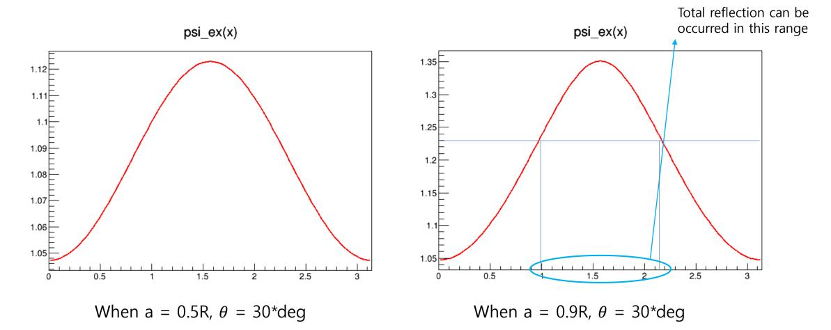
Even if the polar angle is the same, incident angle is changed depending on the position a. For reference, critical angle is about 1.2217.
