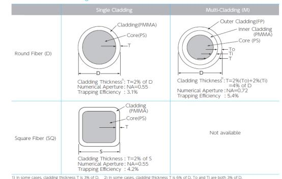
**Cross-section and Cladding Thickness**
