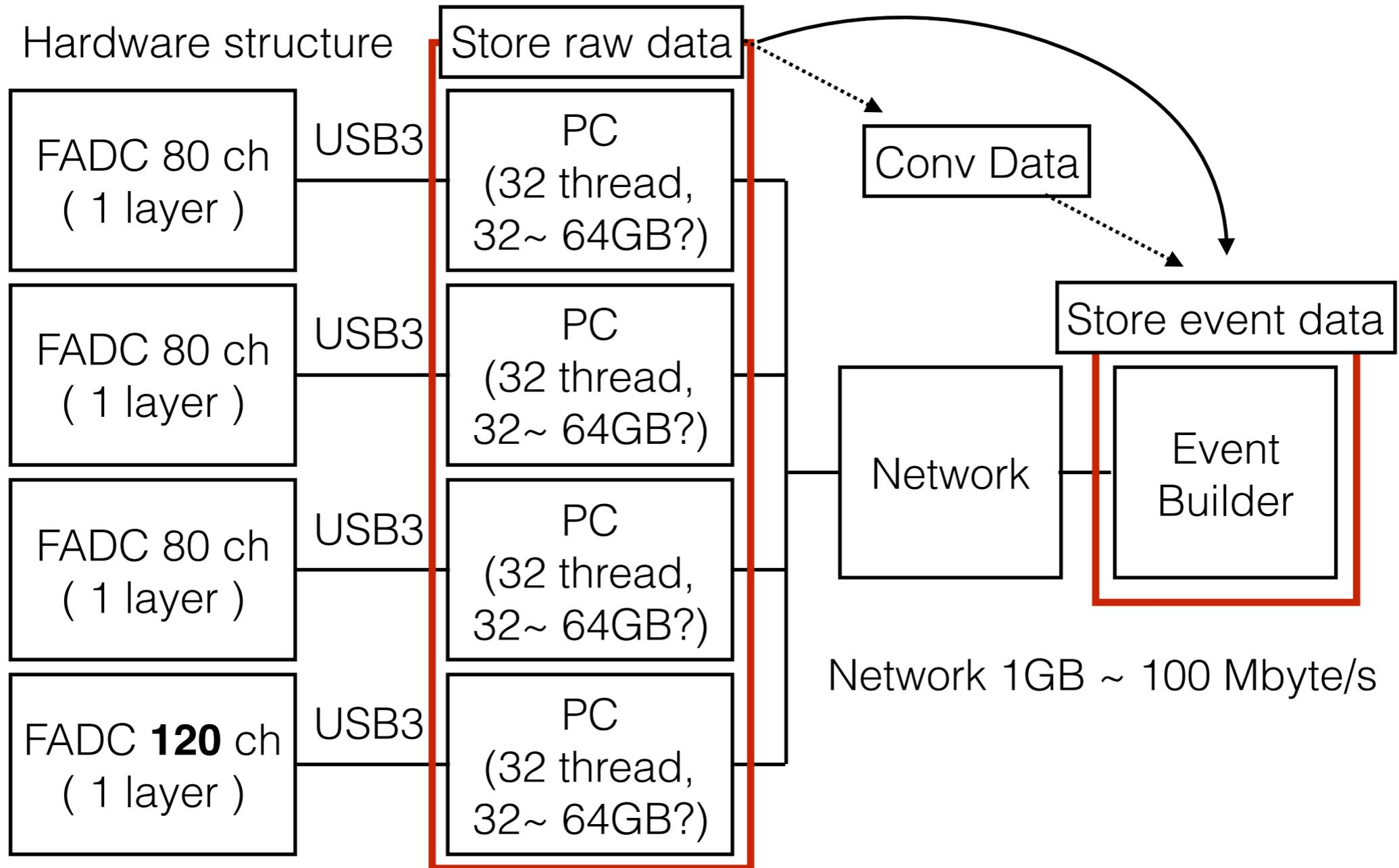
Trigger rate 1k, Number of Hit module 16 (2 modules per One plane),
