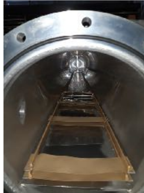
Evacuation by vacuum chamber
