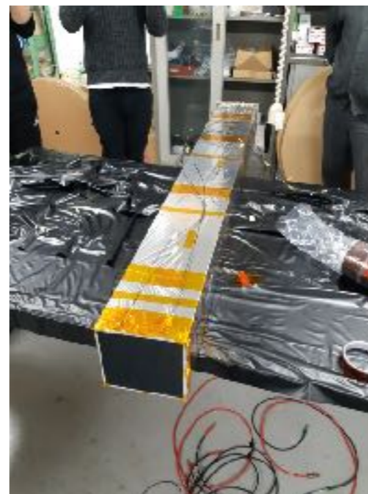
Center Line for beam alignment
