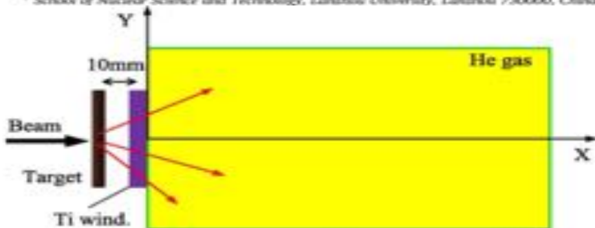
Fig. 3. A simple model for the simulation including a target, a titanium foil and a cylindrical gas cell.
