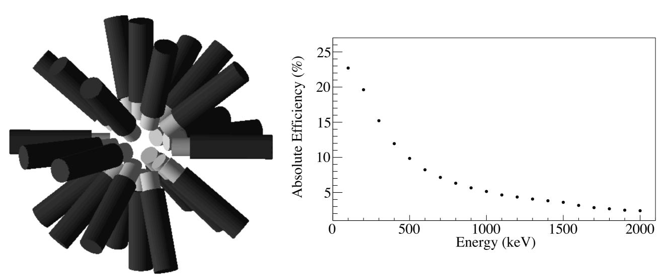
New configuration with mini-ball like geometry.
