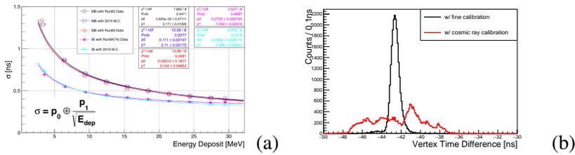
**Figure 2:** (a) The timing resolution of MB and (IB)Inner Barrel. IB provide 1.5 times better timing resolution. (b) Result of timing calibration using  $K_L$  data(black line) and cosmic data(red line)
