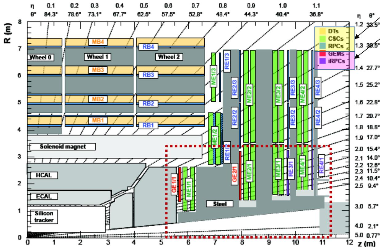
The first ring was left free from RPC due to budget constraints and limited rate capabilities.
