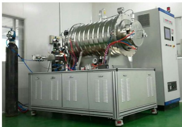
New furnaces for N-doping and infusion study
