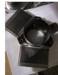
650 MHz 5-cell cavity with waveguide HOM coupler
