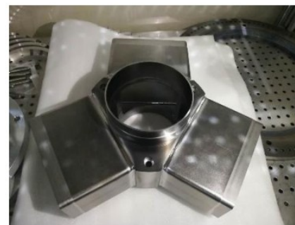
650 MHz 5-cell cavity with waveguide HOM coupler
