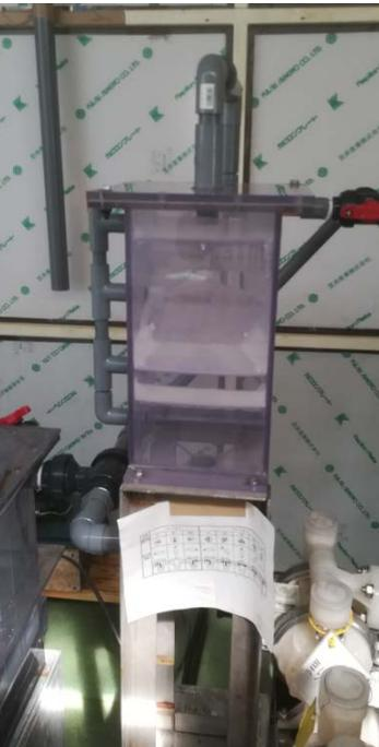
Teflon filter on the acid line to remove H<sub>2</sub>
