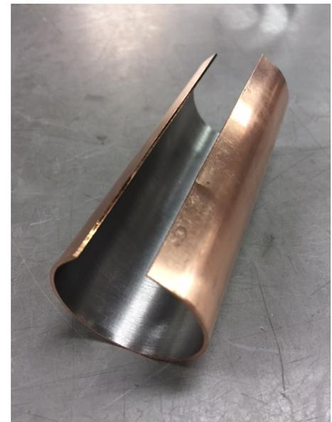
Nb thin film deposited on the inner wall of Cu tube ( $\Phi 35\text{mm}$ ).
