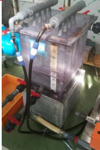
Acid reservoir with Teflon mesh to remove H<sub>2</sub>
