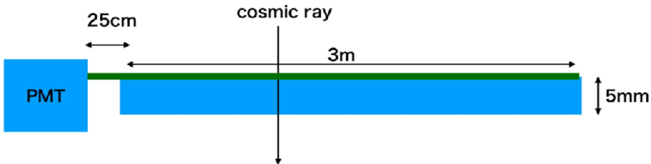
What kinds of pulse we will get when cosmic ray passing through the 5mm-thick and 3m-long plastic scintillator ?
