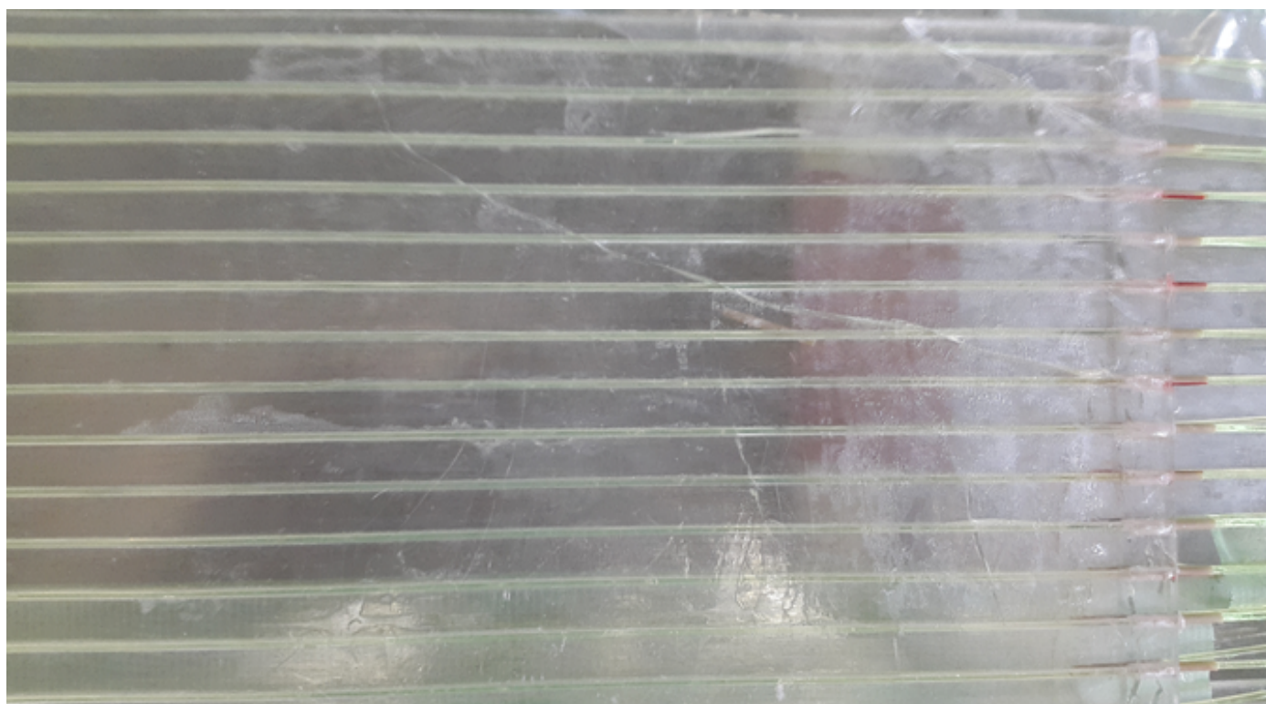
Figure 3.5: Picture of scintillator and wavelength shifting fiber.
