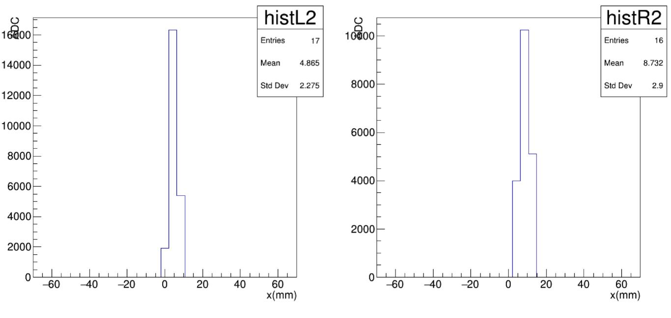
The sigma values of these histograms are used to get the diffusion coefficient D.
