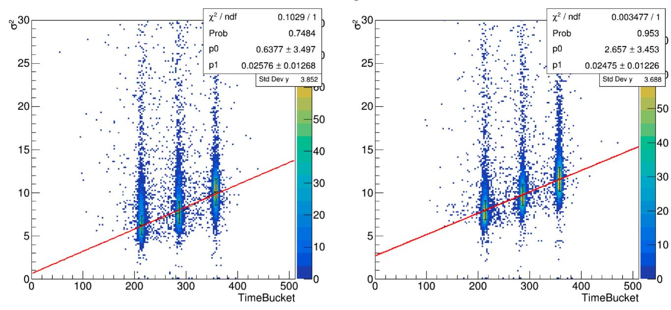
TimeBucket will be changed into the drift distance to get the exact diffusion coefficient.
