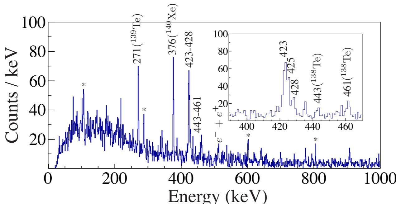
The  $\beta$ -delayed  $\gamma$ -ray singles spectrum and the inset shows the close look of the interest region. 423, 425, and 428 keV photo peaks are candidates for the internal transition. (After the confirmation of the time-different singles spectra.)
