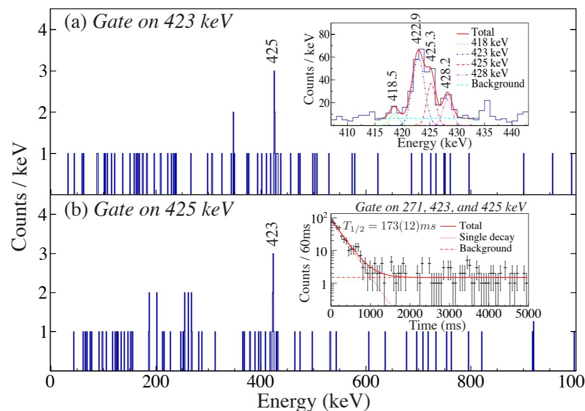
The 423- and 428 keV transitions are coincidence each other. The 428 keV transition does not appear in  $\gamma\gamma$  coincidence matrices. Consider as the transition in  $^{139}\text{Te}$ . No more transition has been assigned.
