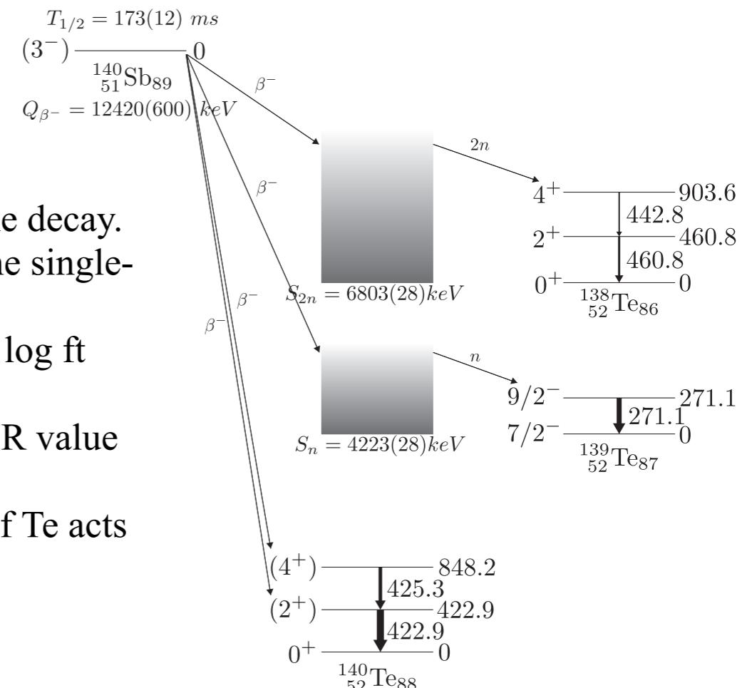
The table represents transition information of the decay. The first forbidden transition is dominant and the single- and double neutron emissions are significant.
