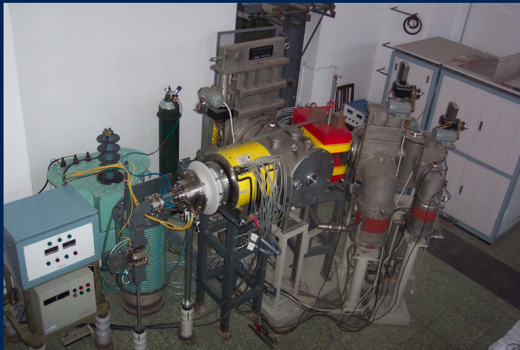
Proton beam with 40 KV and 20 mA
