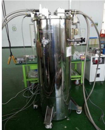
A dewar with cryocoolers (1.5Wx2 at 4K)
