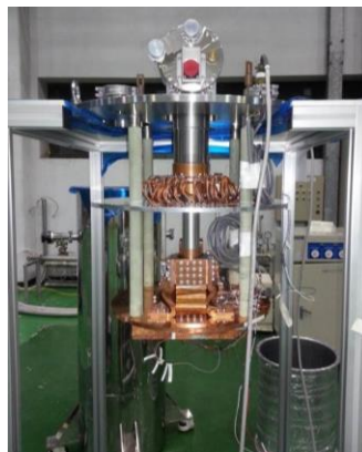
A dewar with cryocoolers (1.5Wx2 at 4K)
