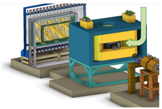
To minimize the area  $\pi$ , K are passing through, we should set the FAC inside the magnet.
