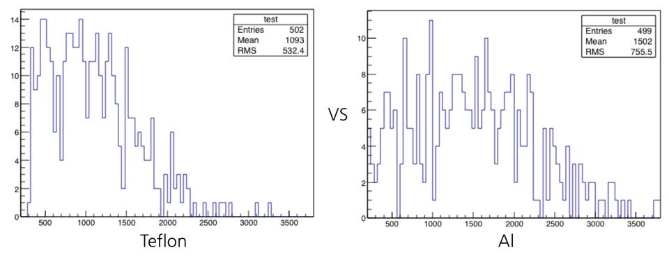
Al reflector shows better light collection (This agrees with another experimental group's simulation result. Al gives shorter flight length for light due to slope.).
