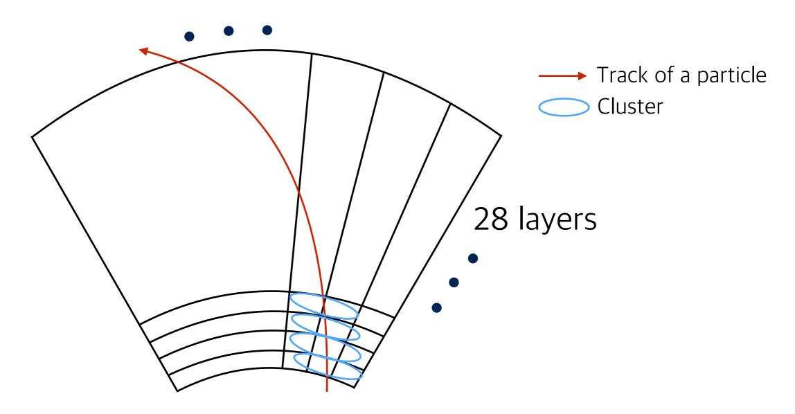
A cluster is defined in only one layer. This means that the number of fired pads in a layer is the size of a cluster
