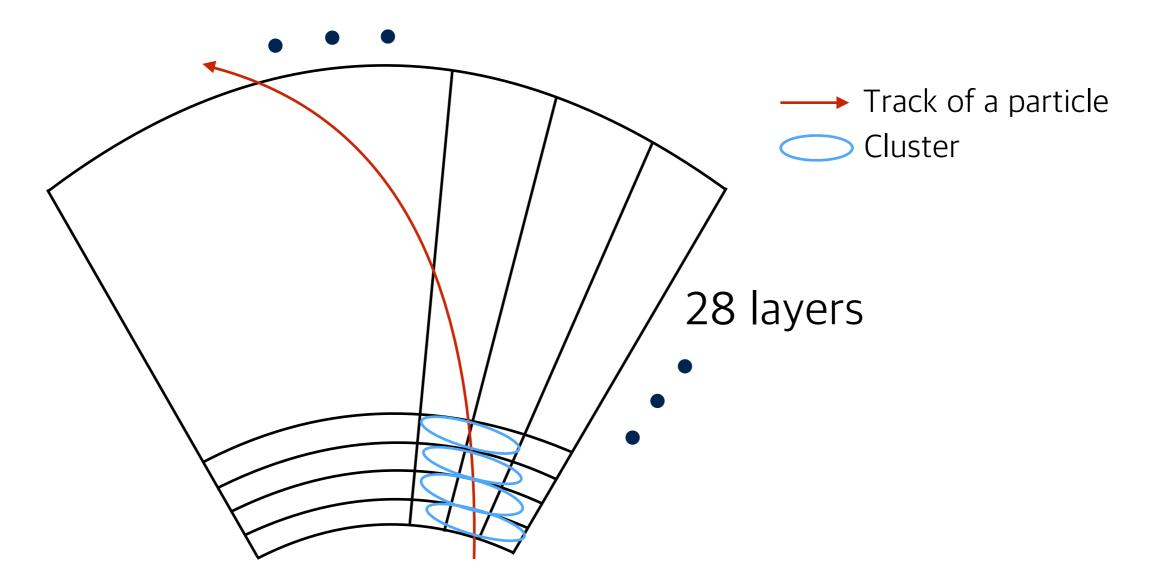
A cluster is defined in only one layer. This means that the number of fired pads in a layer is the size of a cluster
