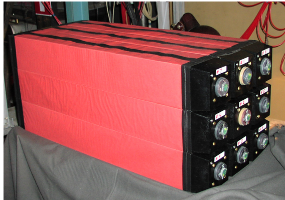
Figure 1.14: 3 \times 3 matrix of prototype Shashlyk modules as they should be employed for the PANDA Forward Electromagnetic Calorimeter.
