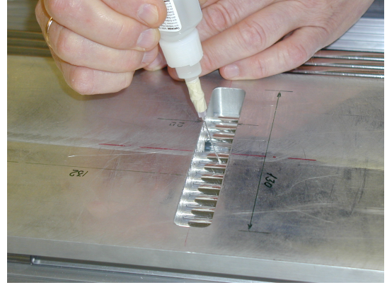
Figure 3.10: The glueing operation of straw tubes in multi-layers.
