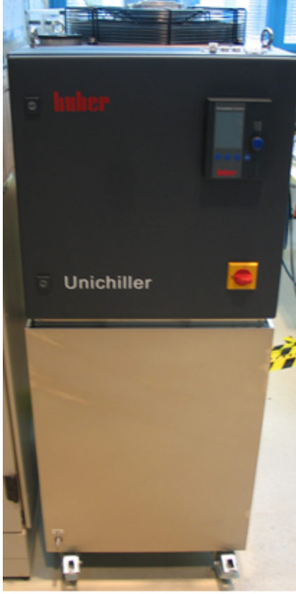
Figure 4.46: Photo of the heater/chiller module Unichiller UHCT with a cooling capability of \approx 10 kW.
