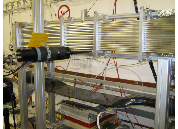
Figure 3.53: Straw tube prototype used at the Institut für Kernphysik at Forschungszentrum-Jülich. Design and construction by IKP-Jülich.
