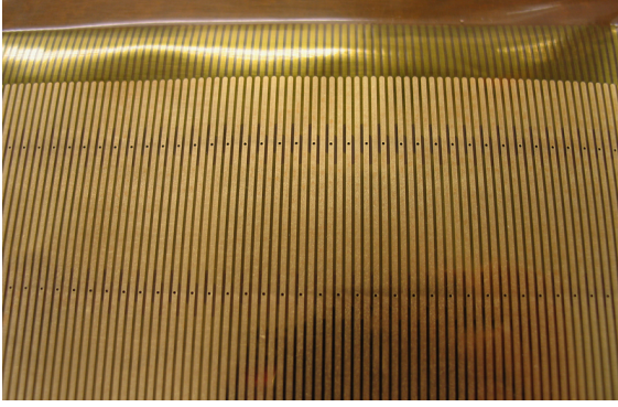
Figure 4.14: Photograph of the strip-line field-defining electrodes. The surface facing the drift volume is shown. The strips of copper metal of 2\mu\text{m} thickness have a width of 1 mm and a gap of 0.5 mm. The holes show the location of the bores used for the gas-distribution system integrated into the walls of the gas-tight vessel of the field cages. On the upper part the picture one clearly recognized the staggered structure of the strip-line electrodes between the front and backside of the foil.
