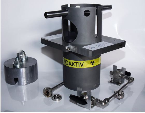
Figure 4.31: Lead-shielded container housing the ^{83}\text{Rb} source. The source is contained in a steel finger that can be attached to the gas inlet via a bypass system. The outer shielding absorbs higher energetic decay photons that are emitted during the decay.
