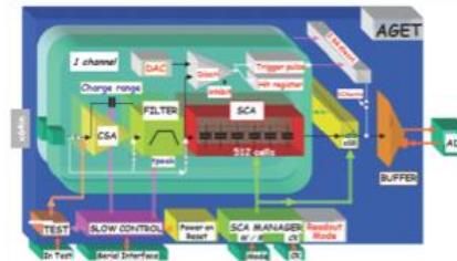
Fig. 2: Block diagram of the AGET chip.
