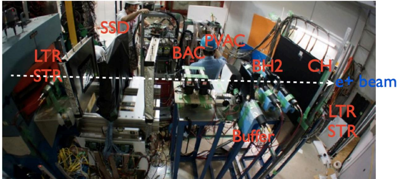
We tested detectors with positron beam at Tohoku University.
