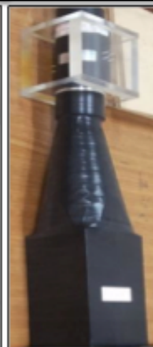
Fig. 4: Detector assembly process. Scintillator BC-408, fish-tail light guide and a photomultiplier tube used.
