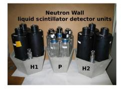
50 closely packed liquid scintillator detectors of three types: H1, H2, P.
