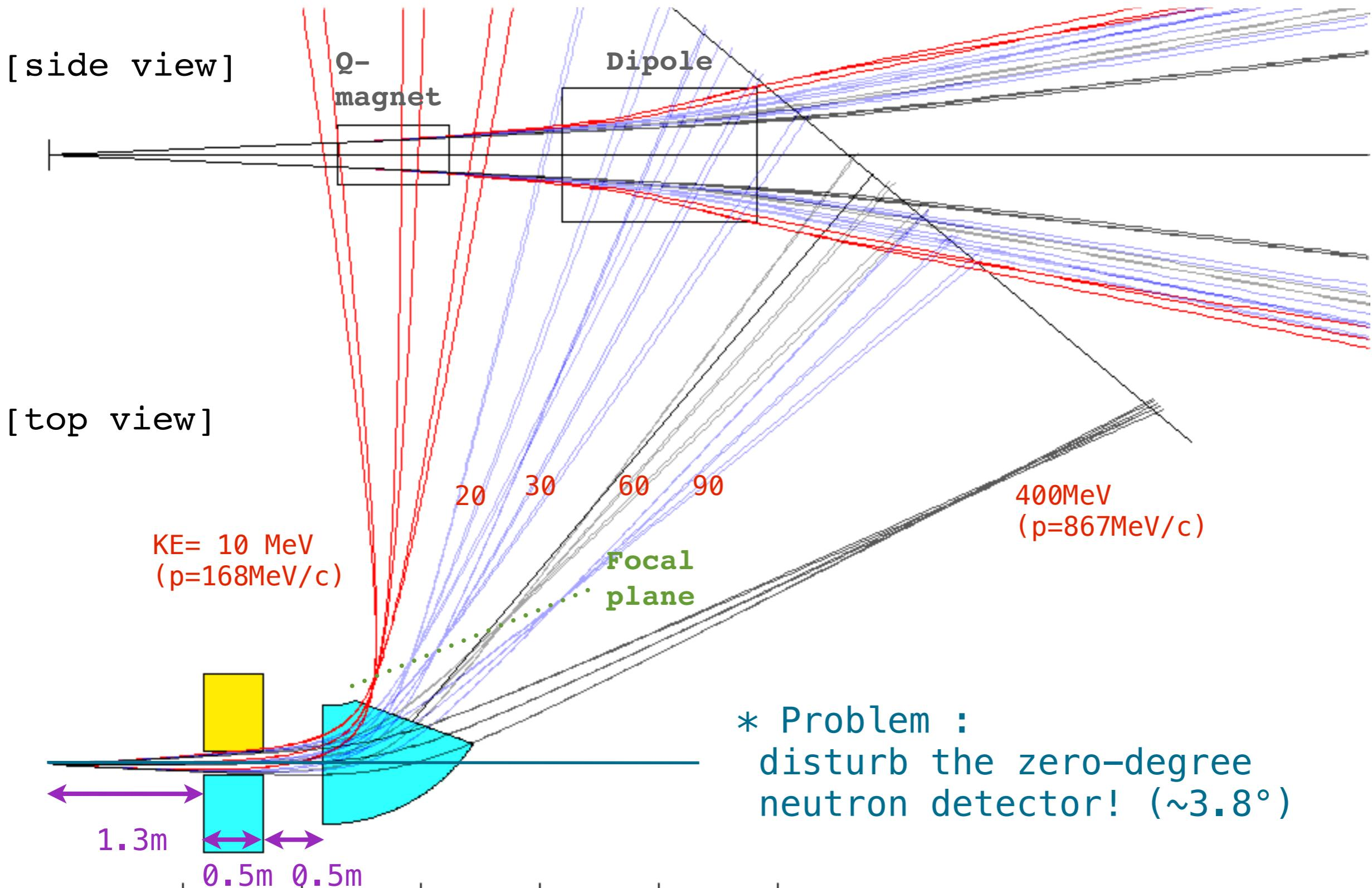
1)  $R=1.0\text{m}$ ,  $B_{DP} = 1.3\text{T}$ ,  $\beta=10^\circ$ ,  $\theta=35^\circ$   $B_Q = 0.5\text{T/m}$  (x-focusing)
