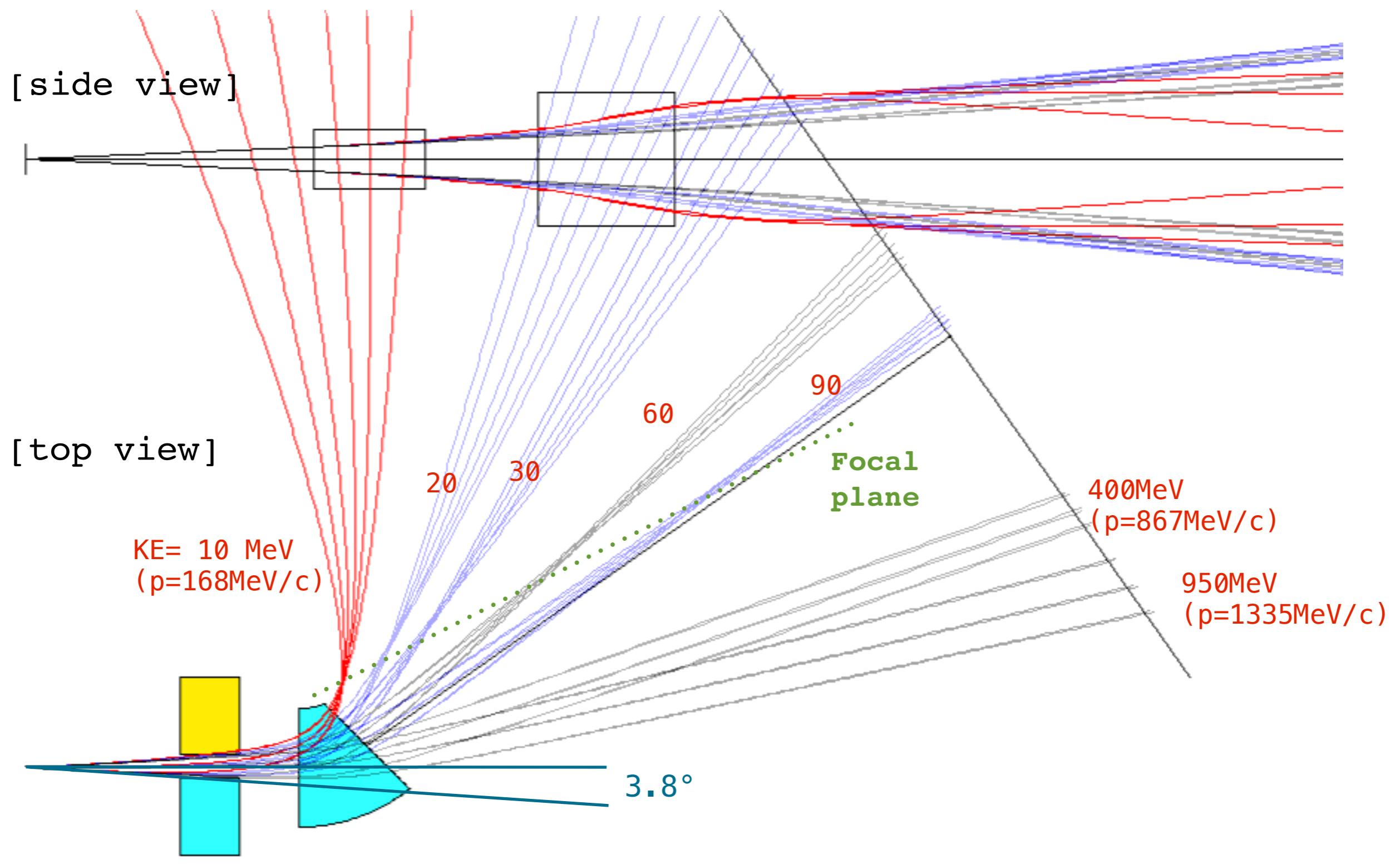
2)  $R=1.0\text{m}$ ,  $B_{DP} = 1.5\text{T}$ ,  $\beta=15^\circ$ ,  $\theta=30^\circ$   $B_Q = 0.5\text{T/m}$  (x-focusing)
