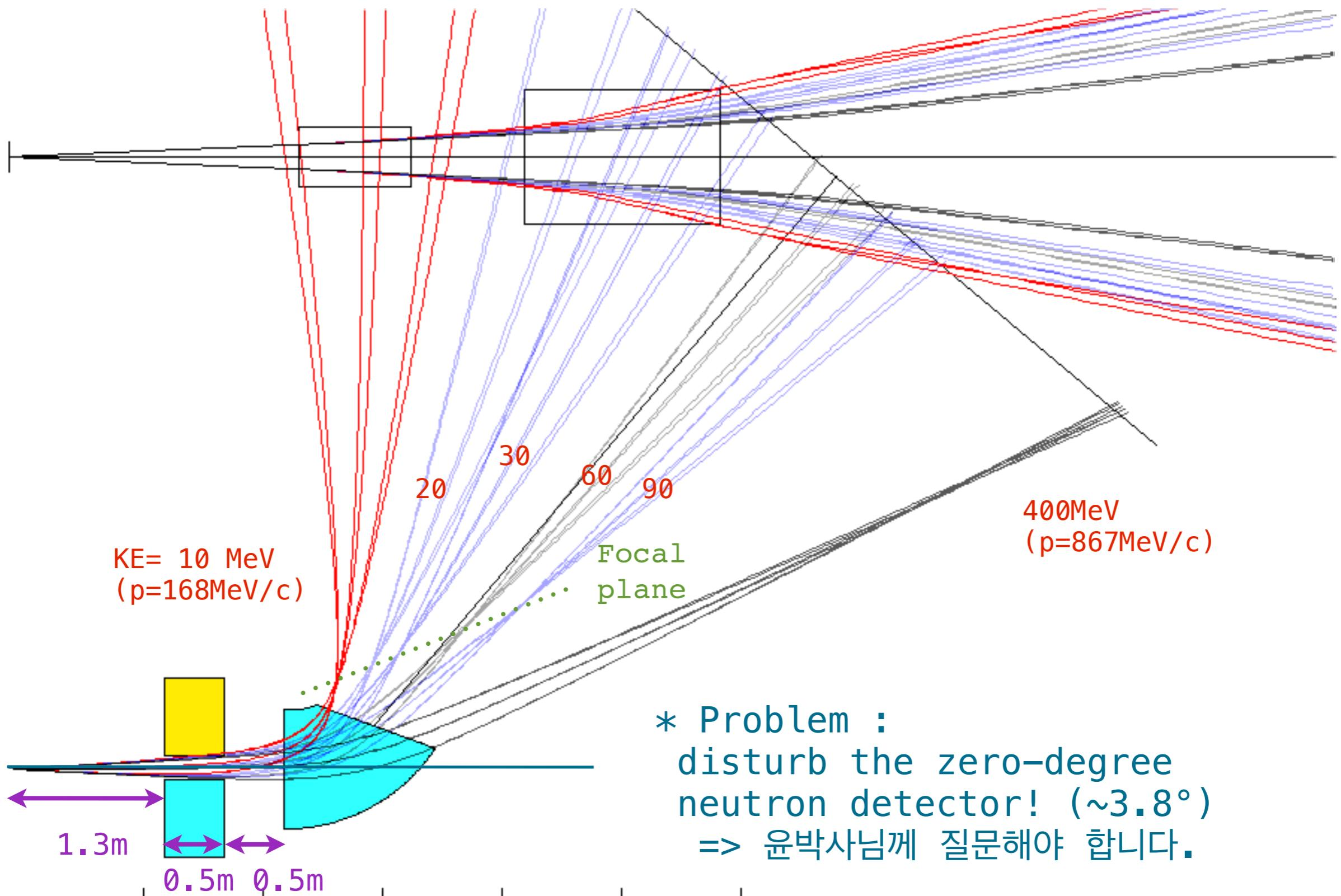
2)  $R=1.0\text{m}$ ,  $B_{DP} = 1.3\text{T}$ ,  $\beta=10^\circ$ ,  $\theta=35^\circ$   $B_Q = 0.5\text{T/m}$  ( $x$ -focusing)
